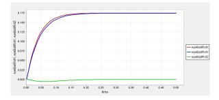
Figure 7: Step response.  $10^{\circ}$  horizontally & vertically. Total saccade duration is more than 160ms, which is far above the observed durations in human subjects (<100ms).
